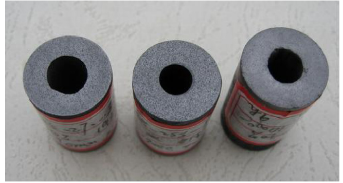
Fig. 5. Photo of the GN-3 laminated ceramic nozzles.
