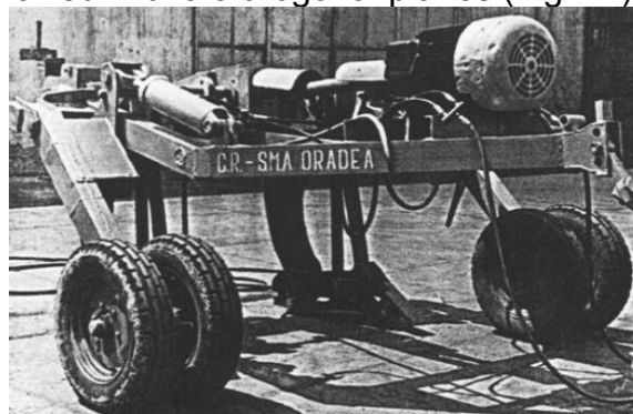
Fig. 14 - Machine for loosening soil with working vibrators operated in two orthogonal planes [4]
