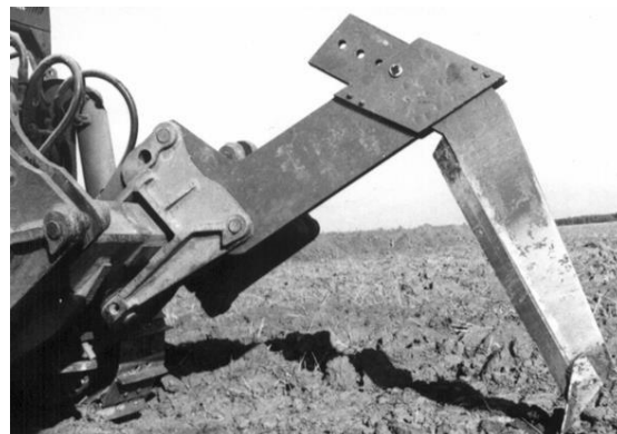
Fig. 9 - Loosening body A-120 for tractor S-1500 LS [1]
