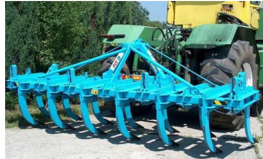
Fig. 16 - Chisel plow and deep loosening equipment PC13-0S [1]
