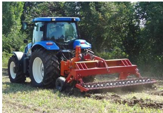
Fig. 17 - Technical equipment with active bodies involved for deep soil loosening EAA [5]
