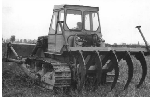
Fig. 12 - Deep loosening equipment 5 bodies active for the S-1500 tractor [2]
