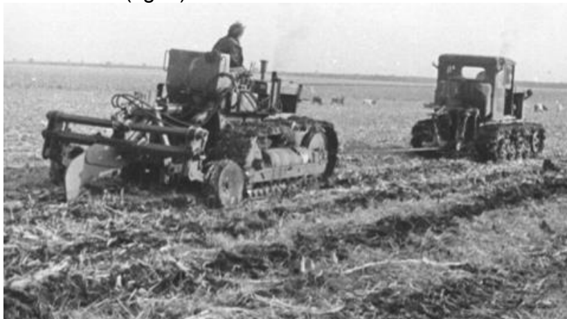
Fig. 7 – Loosening equipment MID-02 with mole device
