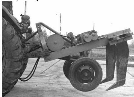
Fig. 13 - Subsolier vibrator SV-2, cu mase rotative neechilibrate [3]
