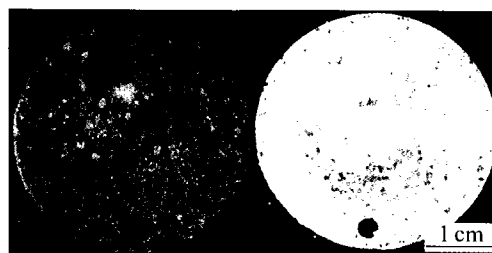
Fig.4 Corroded surface photographs of AZ91 alloy without \text{Na}_2\text{B}_4\text{O}_7 (left) and with 0.6% \text{Na}_2\text{B}_4\text{O}_7 (right) processing
