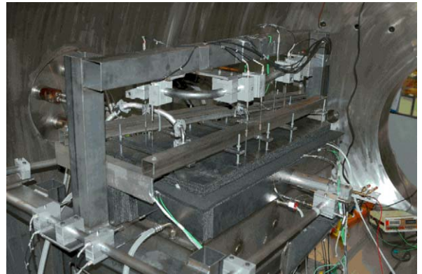
Fig. 26. Test article ready for the thermo-mechanical test (credit IABG).
