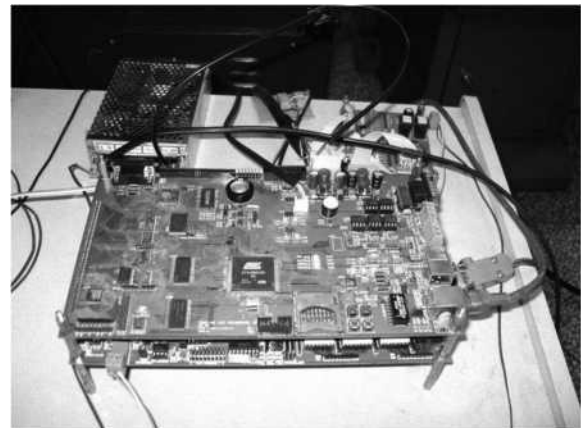
Fig. 9 Hardware setup of the controller. TABLE I
